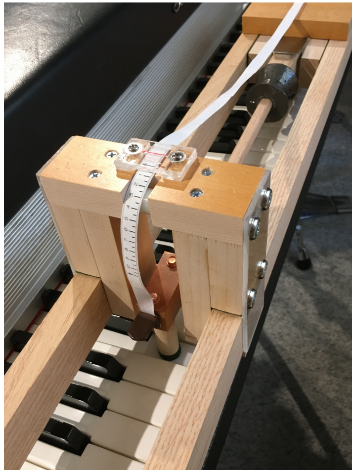
George Mamalakis's "VERA" system for recording precise velocities.
